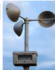
An anemometer measures wind speed.
